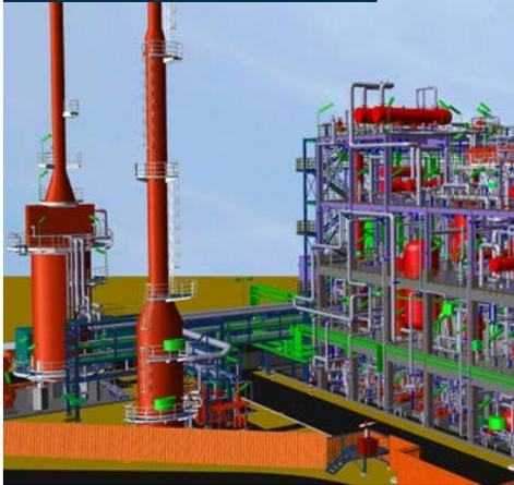
**Conversion of a propane deasphalting plant (PDA plant) built by EDL in 2011 to produce deasphalted oil from vacuum residues by extraction using liquid propane.**
